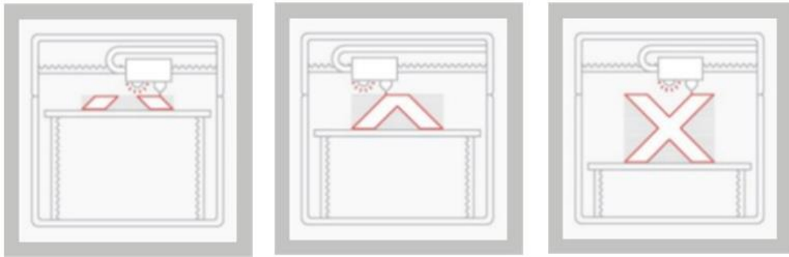
Figure 1.12. Material Jetting 3D printing process
