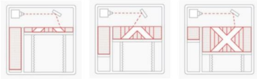
Figure 1.8. SLS printing process
